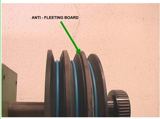
These pulleys are suitable to return and deflect the direction of wires or cables when moving, the root diameter on groove is 120 mm. The pulley has the ceramic or Ertalon groove for long life of surface. All pulleys are mounted on double bearing.
